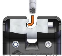
After that the towing rope is clamped **slightly** by the set screws. To reach the set screws the plastic housing can be turned on the clamp by roughly 45°:
